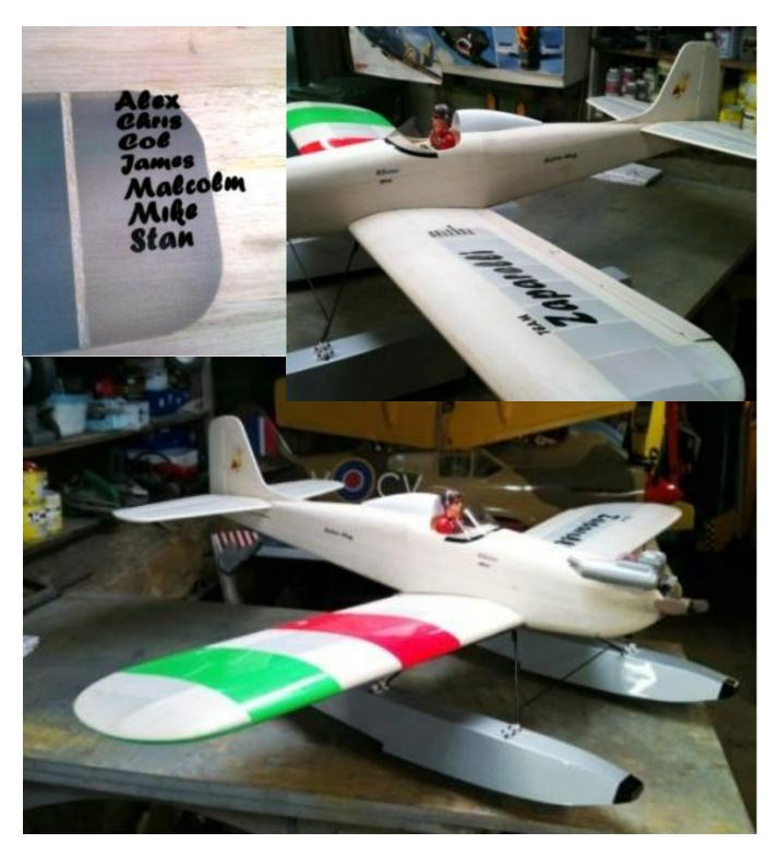
We covered the plane with a mixture of Solartek and scrap Monocote. The Solartek is a natural fabric finish and the Monokote is in the Italian colours to denote its Pizza house home.
